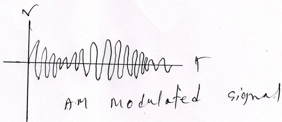
AM (Amplitude Modulation) is a type of analogue modulation where the information of the message signal is stored in the amplitude of the carrier signal. The frequency range of AM is 535 to 1605 kHz which is less as compared to other modulation techniques.
