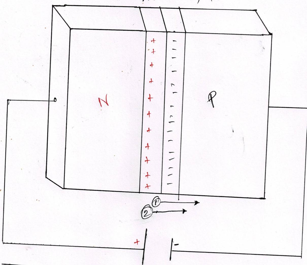
① Battery induced electric field | ② Built in electric field.
