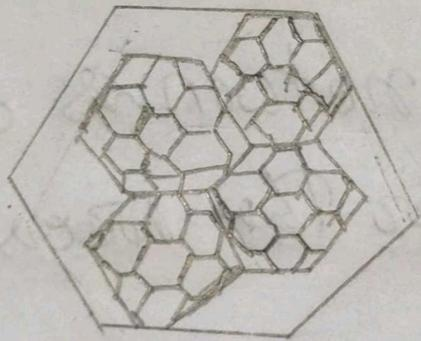
A cell pattern using 34 cells in a cluster.
