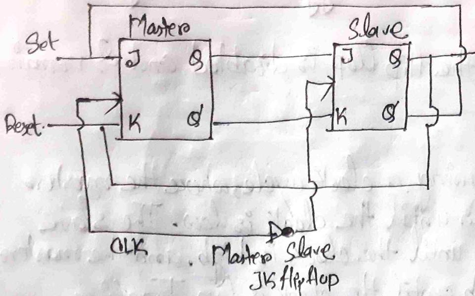
When the clock pulse goes to 1, the slave is isolated; J and K inputs may affect the state of the system. The slave flip flop is isolated until the CP goes to 0. When the CP goes back to 0 information is passed from the master flip-flop to the slave and output is obtained.
