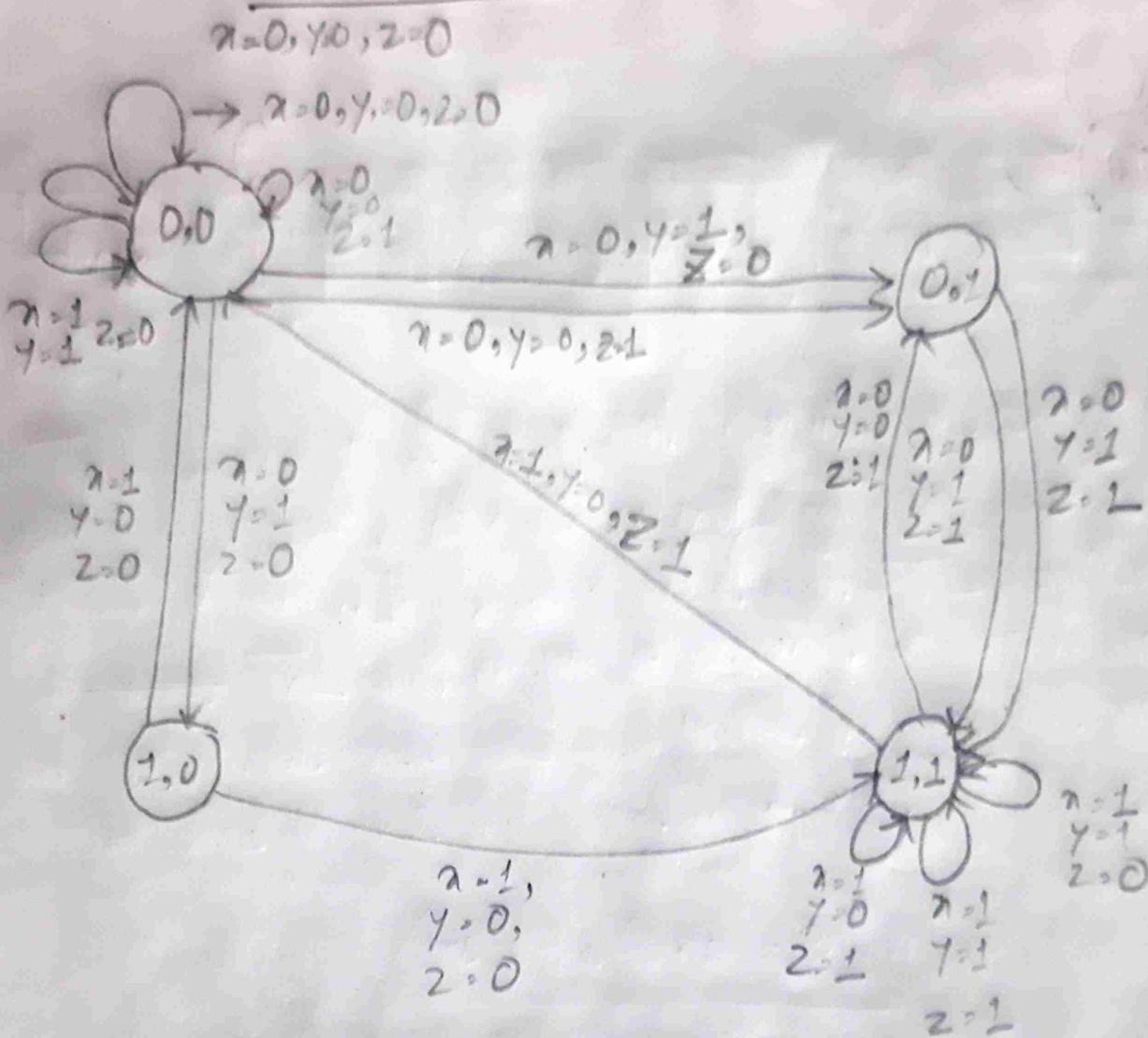
$x, y = \text{input } \& z = \text{output}$
