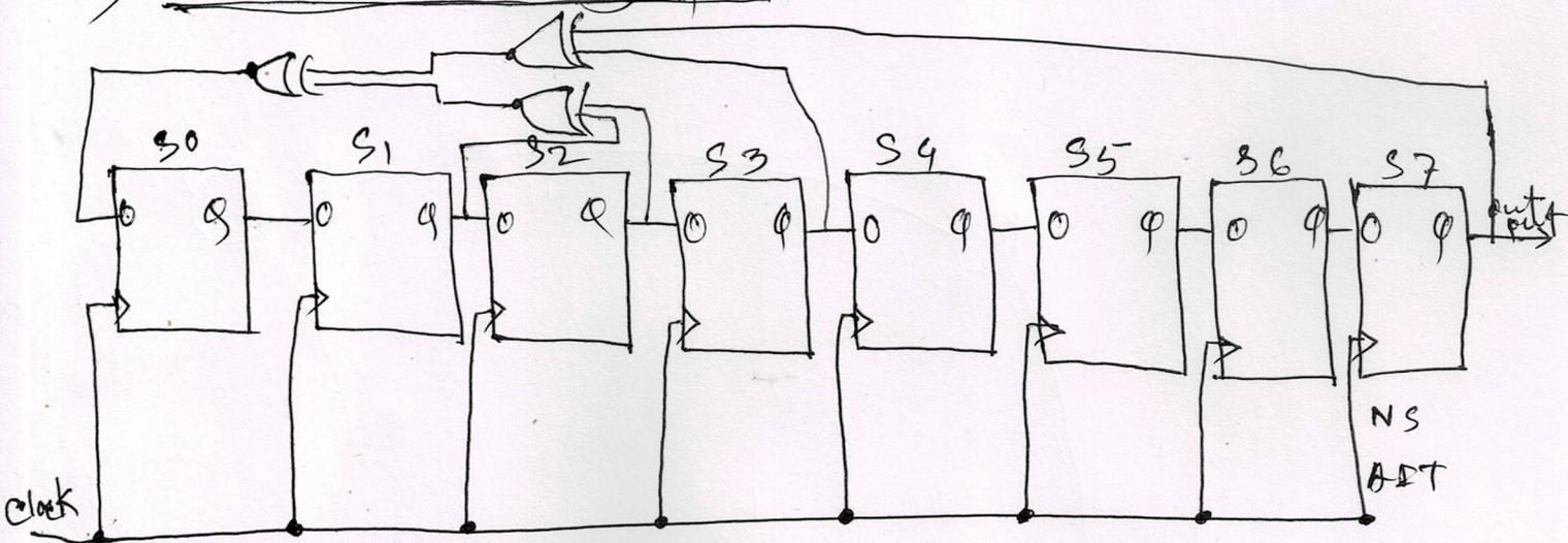
The following register is a 8-bit serial register.
