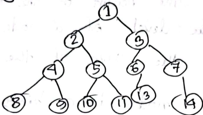
Binary tree Representation - A binary tree is represented by a pointer to the top most node. (commonly known as the root) of the tree.
