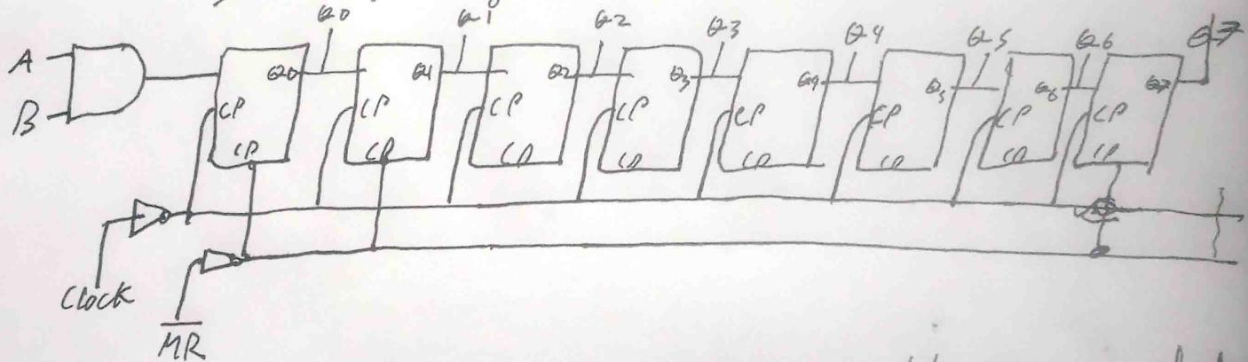
8 bit serial register allows data to be shifted in and out one bit at a time in a serial manner. One clock period is  $(1/2)$  micro-s = 0.5 microseconds.
