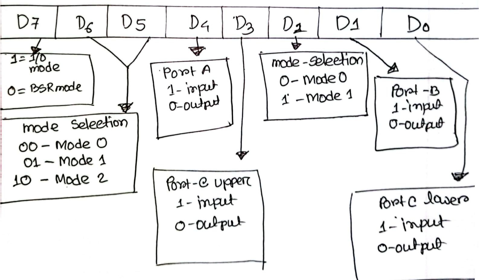
in this specific control word, Port A is configured in mode 1, port B is configured in mode 0, and Port C is configured in mode 1. keep in mind that the exact interpretation of these modes and the functionalities they represent would depend on the specific application and requirements for the 8255 chip's operation.
