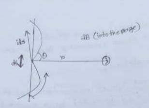
consider a current carrying wine in in a specific direction as shown in the above figure. Take a small element of the wine of length ds. The direction of this element is along that of the current so that it forms a vector i ds. To know the magnetic field produced at a point due to this small element, one can apply Biot-Savarts law. Let the position vector of the point in question drawn from the aurment element be n and the angle between the two bot. Then,
