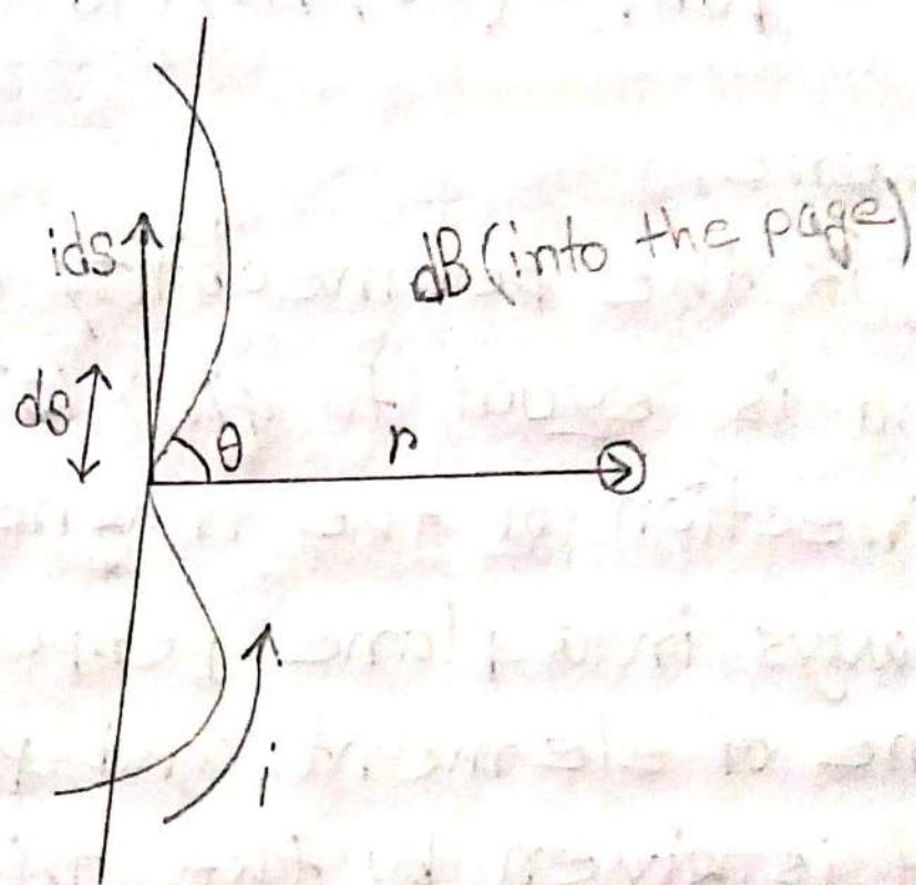
consider a current carrying wire in a specific direction as shown in the above figure. take a small element of the wire of length  $ds$ . The direction of this element is along that of the current so that it forms a vector  $i ds$ . To know the magnetic field produced at a point due to this small element, one can apply Biot-Savart's Law. Let the position vector of the point in question drawn from the current element be  $r$  and the angle
