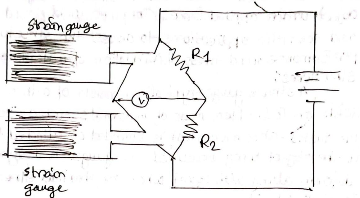
Strain gauges offer several advantages, such as high sensitivity advantages, such as high sensitivity, accuracy, and versatility. They can be used to measure various types of strains, including tensile, compressive, and shear strains. Strain gauges find applications in fields like structural engineering, aerospace, automotive, biomechanics, and material testing, where pre-strain measurement are necessary for design analysis, and quality control purposes.
