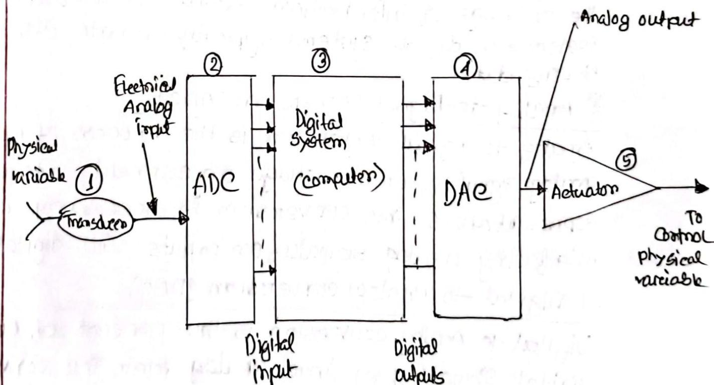
Analog interfacing involves the connection and communication between analog devices or systems. It refers to the process of converting analog signals from one form to another, enabling compatible and interfacing between different analog devices or components.
