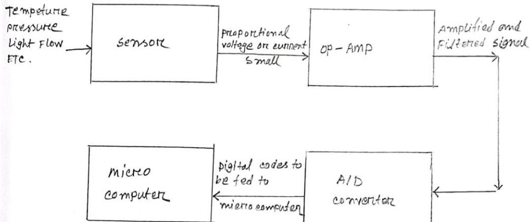
The basic concept of analog interfacing involves several key elements:-
