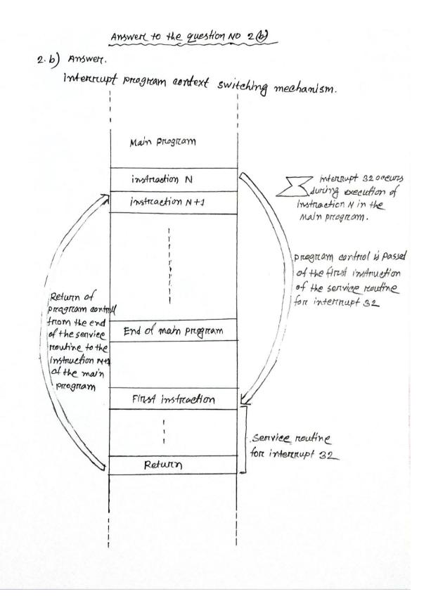
when an interrupt signal occurs, the mps must suspend what it is doing in the main part of the program and pass control to a special routine ISR (the interrupt-service routine) that performs the function required by the external device.
