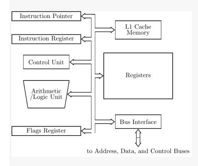
The central processing unit (CPU) is the heart of a computer system, and it is responsible for executing instructions and processing data. The main components of a CPU are the Arithmetic and Logic Unit (ALU), the Control Unit (CU), and the Registers.
