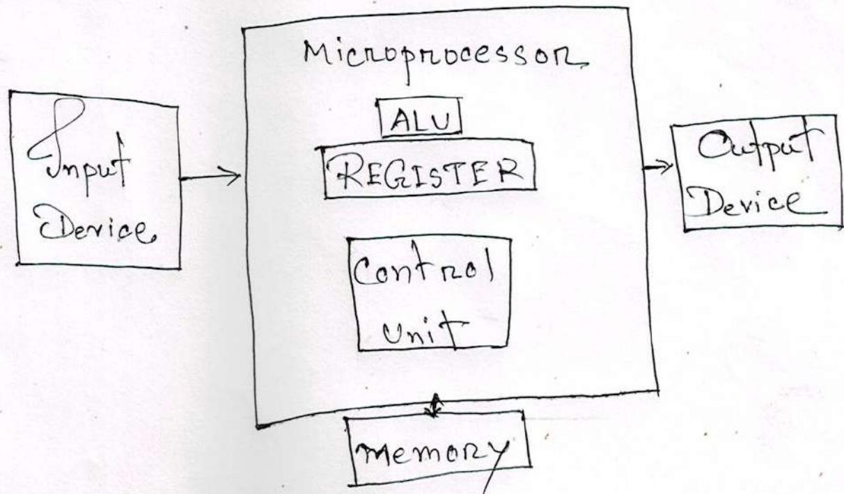
Block Diagram of Basic Microcomputer.
