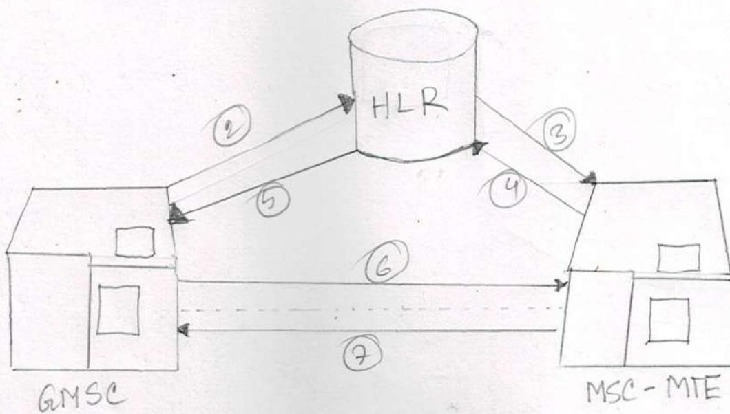
Hand over call: In cellular telecommunication, the terms handover or hand off refers to the process of transferring ongoing call or data connectivity from one base station to the base station. When a mobile moves into the different cell while the conversation is in progress. Then the MSC (Mobile Switching center) transfer the call to a new channel belonging to the new base station.
