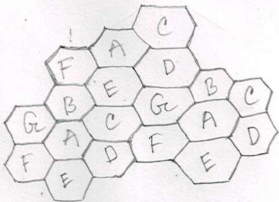
Fig: frequency Reuse.
