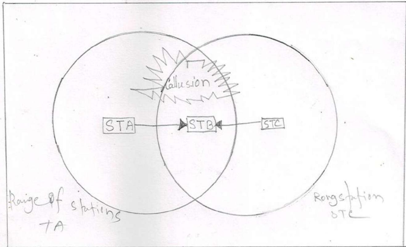
\* Suppose that three out of three stations labelled STA, STB and STC are transmitting while STA is receiving. The stations are in a configuration such that the two transmitters STA & STC are not in the radio range of each other. The above diagram shows that station STA starts transmitting to station STB. The frames received by STC are garbled and collision occurs. The situation is known as the hidden terminal problem.
