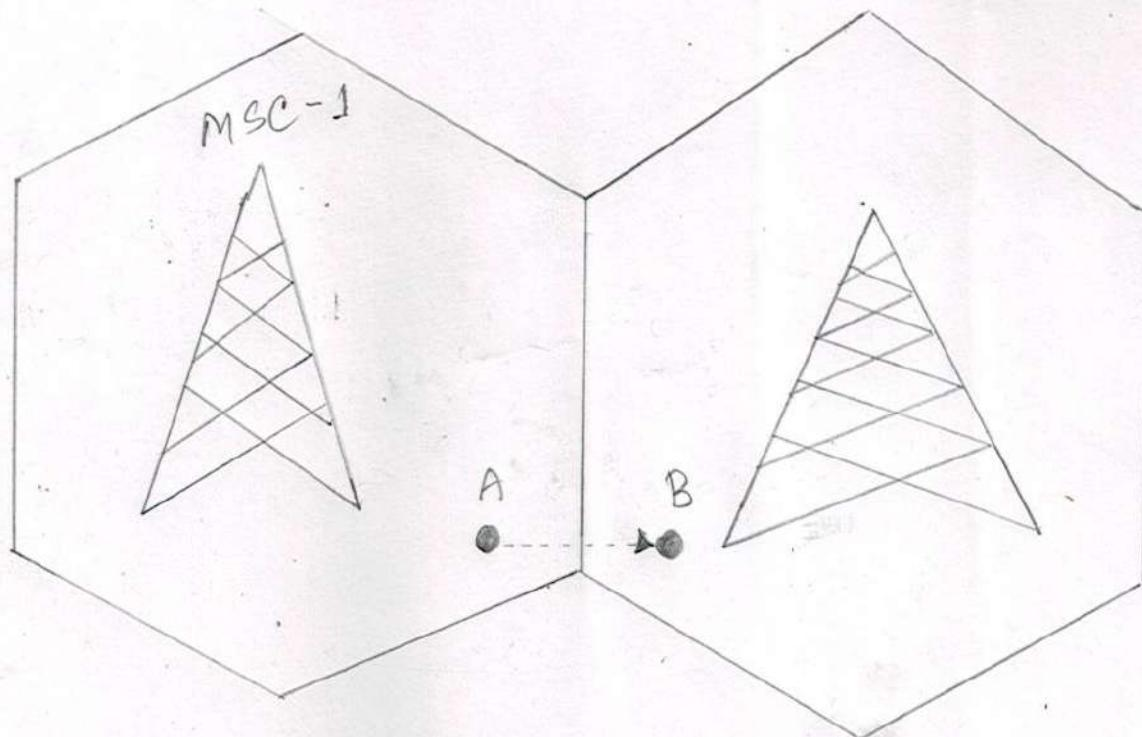
When a mobile user moves from one cell to another cell then BSC 1 signal strength loses for the mobile user A & the signal strength of BSC 2 increases and the ongoing call or data connectivity for mobile user goes on without interrupting.
