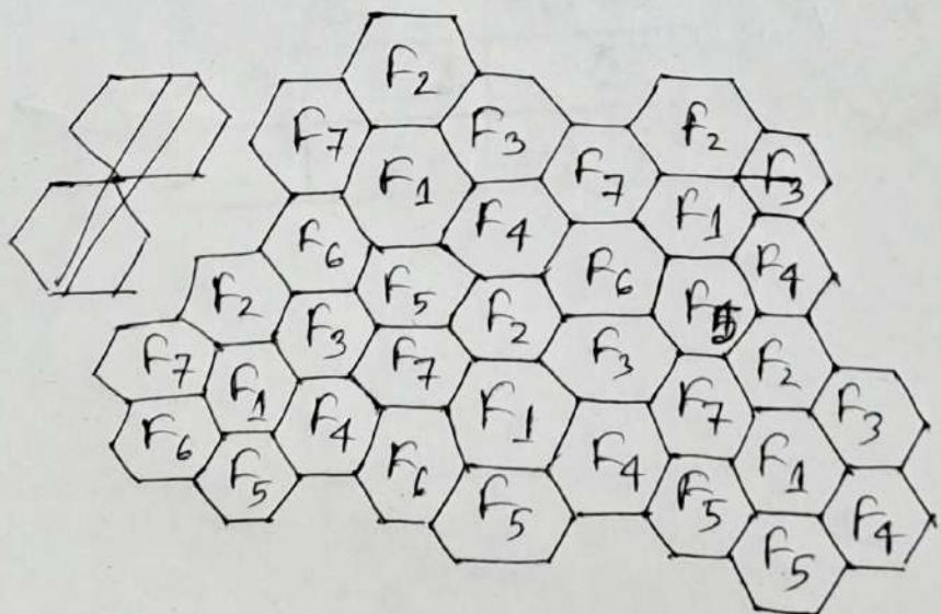
Each cell is generally 4 to 8 miles in diameter, with a lower limit around 2 miles.
