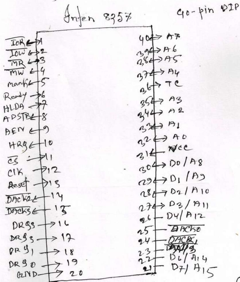
Fig: physical pin diagram of Intel 8257.
