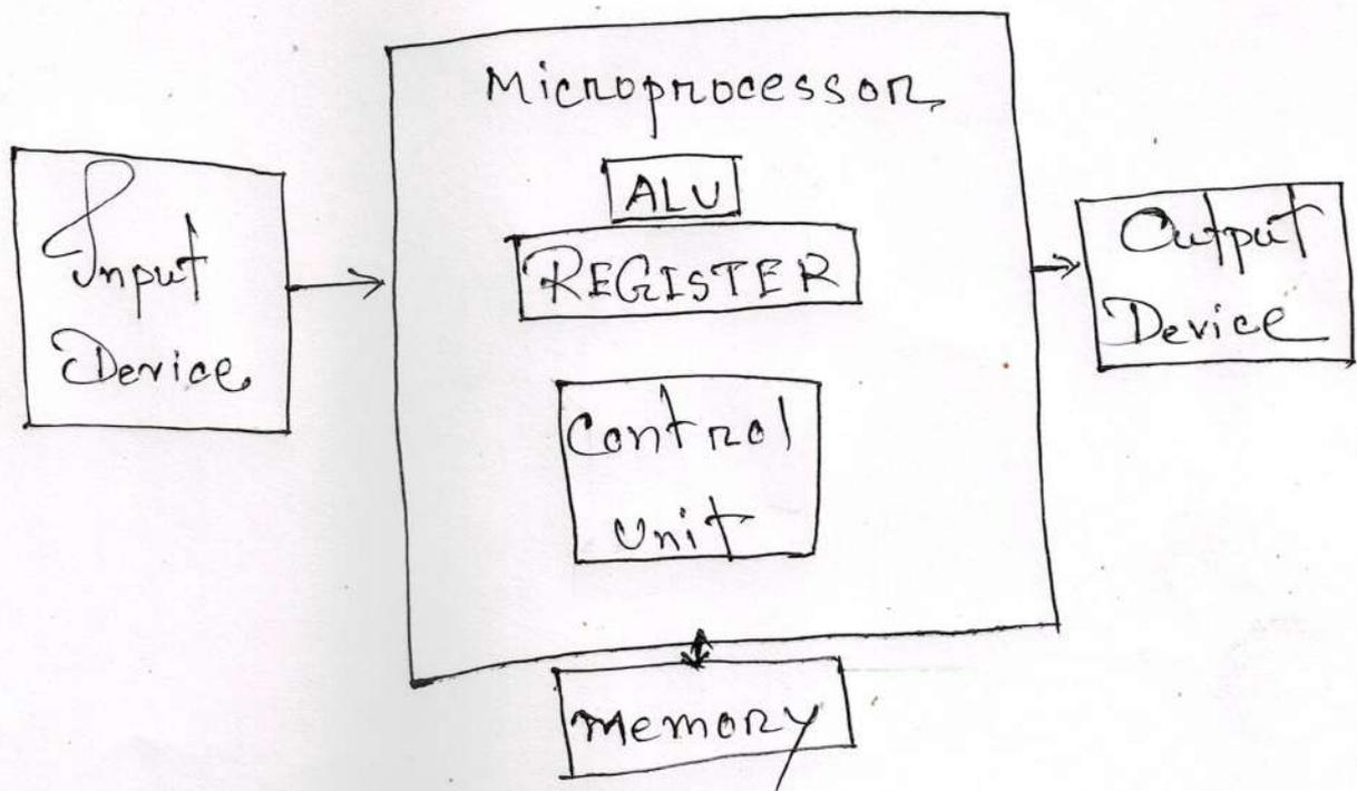
Block Diagram of Basic Microcomputer.
