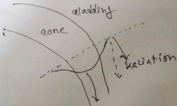
The part of mode which is on the outside of the bend is required to travel faster than that on the inside so that a wavefront perpendicular to the direction of propagation is maintained.
