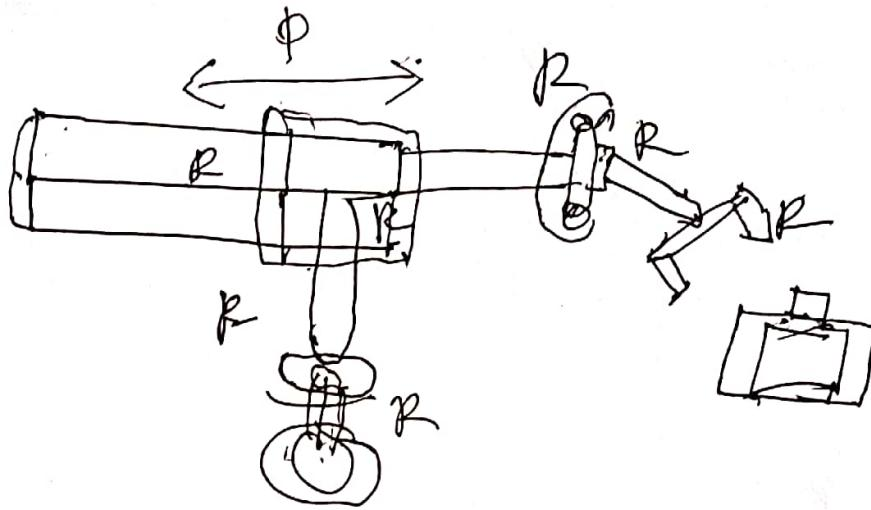
States: Real-valued coordinates of robot joint angles; parts of the object to be assembled.
